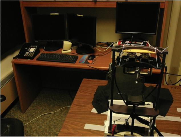
Figure 1: The experimental scene included the display eyepieces from our nVisorSR mounted on a chin rest (near right), a monitor to serve as the real world in the nVisorST's line of sight (far right), and two monitors to show the experimenter what image was being sent to the nVisorST (far left).
