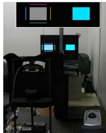
Figure 12: The color perception experiment showed side-by-side patches to be matched. The physical barrier shielded the user's view of the target (left) so that it was seen only through the AR display. With the Glasstron on the chin rest and both sides of the monitor and user performance of 62.5% accuracy, the threshold for better performance than guessing on a four-alternative forced-choice task. The inset shows an example initial target and a reference.
