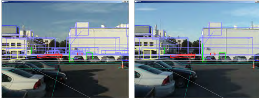
Fig. 9 Left: Showing all information and labels in the database can overwhelm the user and prevent a Marine from achieving SA. Right: Our information filter uses semantic keys and the concept of area of operations to limit the information shown, which enables the user in this case to discern the location of enemy tanks – spotted by another user – much more easily.
