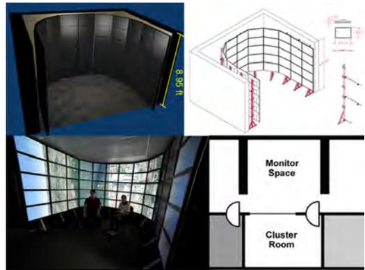
Figure 1: *Left to right, top to bottom:* A 3D sketch of the wall layout, the support structure design, a photo of the wall display Google Earth, and a floorplan of the laboratory space occupied by the monitor wall and the cluster that runs it.
