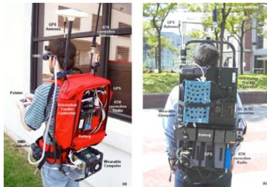
Fig. 5: Experimental mobile AR systems of NRL (left) and Columbia (right) in 2000.
