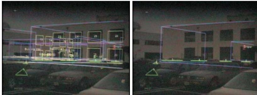
Fig. 3 The need for information filtering. *Left:* "raw" data, a confusing clutter of many different labels and objects. *Right:* filtered output draws the foreground building for context, the path the user is following, and a potential threat. (Recorded by a video camera looking through the head-worn display.)
