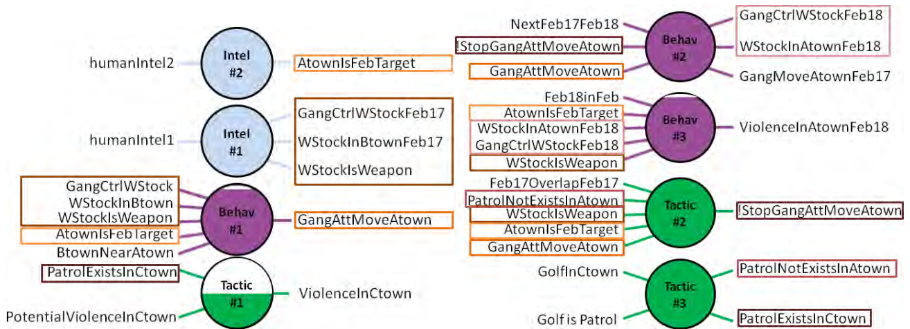
Figure 2. An illustration of our algorithm on a scenario that fits with our intended application. This shows the algorithm’s progress through the matching of antecedents (leading into nodes from the left) and consequents (emerging to the right from nodes), just before the graph is built. The boxes are used for illustration of matches; this view is not shown to users.
