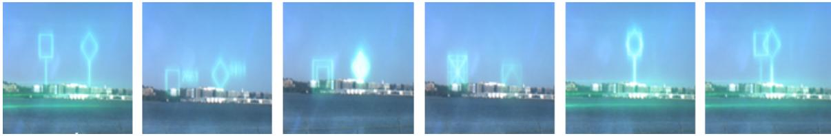
Figure 1: Views through the HMD of several representations used in this study. Left to Right: Ground Plane, Distance Label, Virtual Tunnel, Virtual Wall (all from the Zone Identification task), Ground Plane 50% overlap, Ground Plane 100% overlap (both from the Proximity task).
