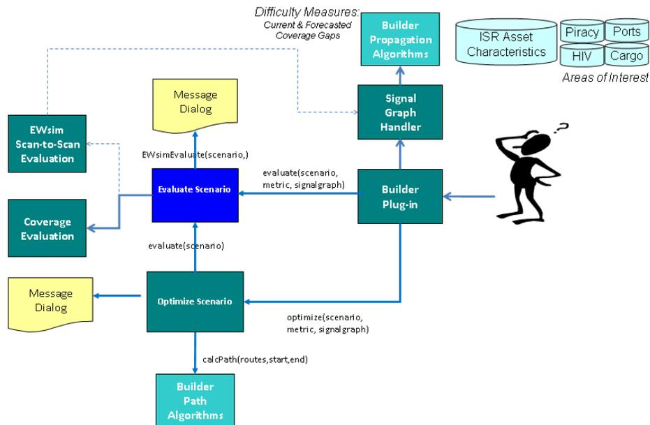
**Figure 1: Sensor Allocation Tool Components**
