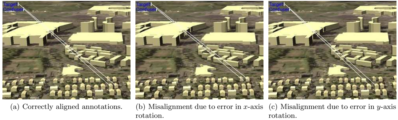
Figure 1. The effects of registration errors. Building names are indicated by the label at the top left of the screen and a call out line which points to the building. A heading error of 1^\circ causes the callout lines to point to the wrong buildings.
